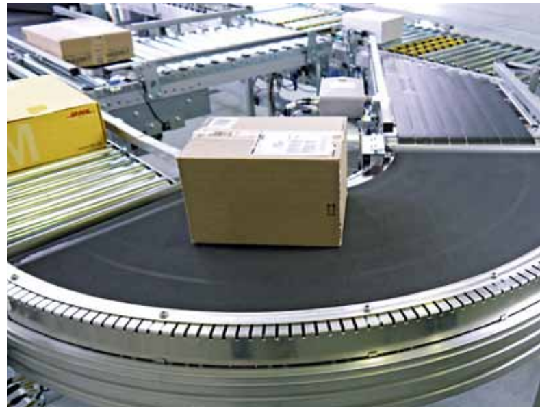
Curved conveyor in a distribution centre.
