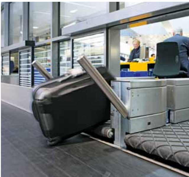
Collecting belt in check-in area of an airport. The flatness of the belt type here ensures that the goods can be discharged to the side smoothly, even on wide belts. Flame-retardance is a “must” in modern airports.
